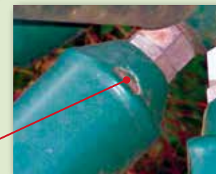
► No under-film corrosion after 12 years.
