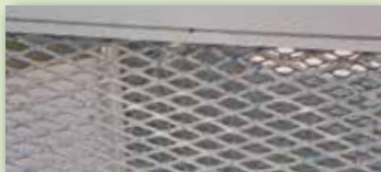
▼ Deteriorated polyester coating in 1996 after 6 years.
